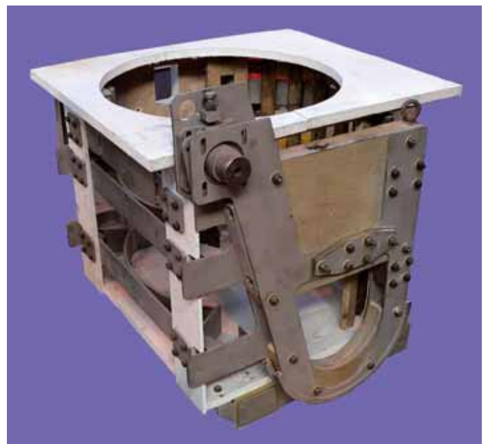
Fig. 8: Induction crucible furnace featuring DURATEC-XP
