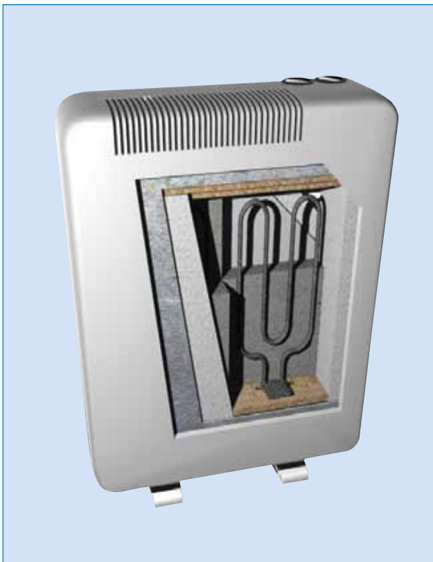
▲ Heat storage stove
